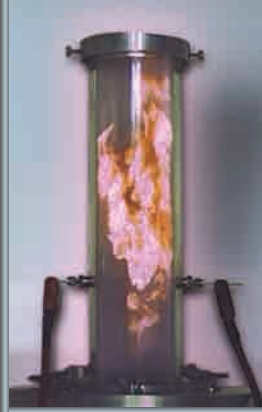
Minimum Ignition Energy (MIE) test of Coal Dust
